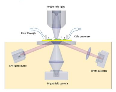
The detector measures the SPR response at each pixel and maps them into a SPR image. At every pixel, a sensorgram is recorded, thus providing much more localized information. SPRM makes it possible to study heterogeneous surface binding and interactions
