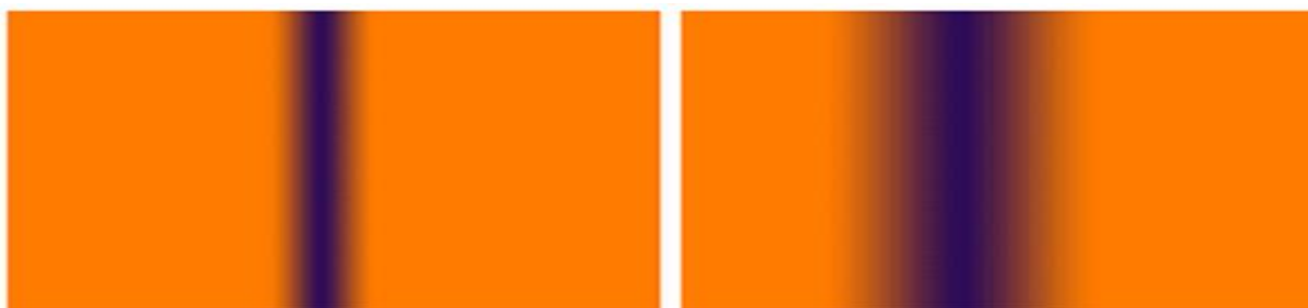
Figure 3. A good metal film gives a clean and straight SPR dark line in air (left) and solution (right).
