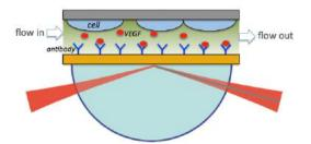
FIG. 1 Experimental setup with cancer cells immobilized onto the ceiling of the BI-SPR flow channel. Cancer cell excretions were detected by capture proteins immobilized on the sensor surface.
